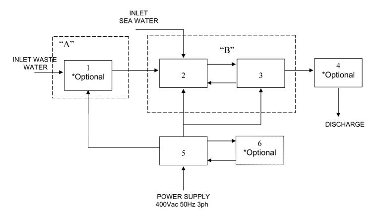
Figure 4.1: Flow chart of the operation of BLUE SEA
